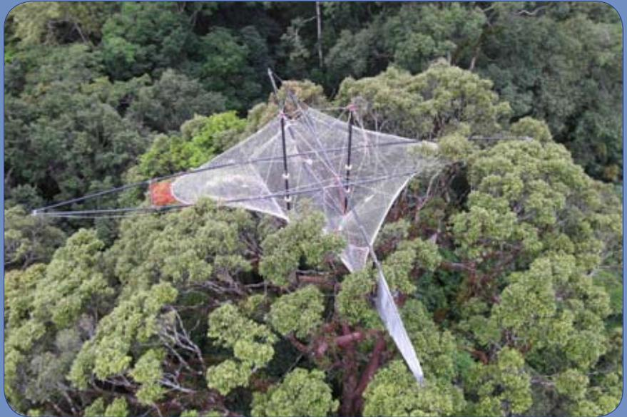
The "Canopy Star" is a mobile tree platform, made of carbon fibre and nets, with a span of about 12 metres
